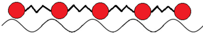
Figure 2: Representation chain of particles upon a substrate potential, incommensurate to the potential. van den Ende J, de Wijn J.A. The effect of Temperature and Velocity on Superlubricity 5 Figure 1.
