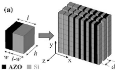
Figure 4: Meta-transmit array showing aluminium doped zinc-oxide (black) and silicon dielectric (grey).
