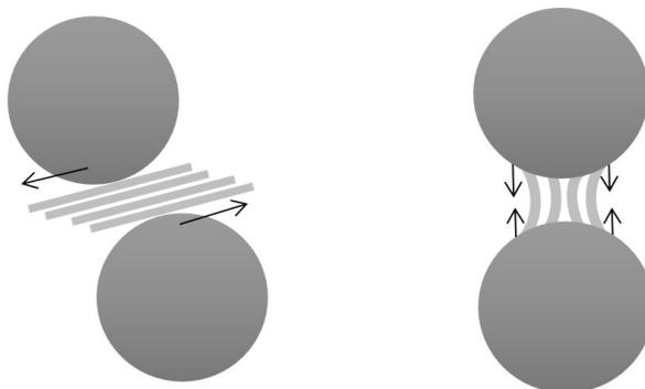
Figure 2: Ball milling for 2D nanosheet production through (a) shear force and (b) compressive force induced exfoliation of layered crystals.
