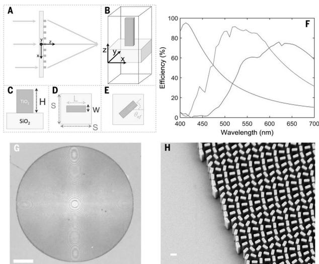
Figure 5: A-E - Schematic of lens and dimensions of the  $\text{TiO}_2$  nanofin. F - Efficiency as a function of wavelength as per simulation of three different nanofin dimensions (In order from left,  $\lambda = 405 \text{ nm}$ ,  $\lambda = 532 \text{ nm}$  and  $\lambda = 660 \text{ nm}$ ). G - The metalens designed at a wavelength of  $660 \text{ nm}$ . H - SEM image of the metalens.
