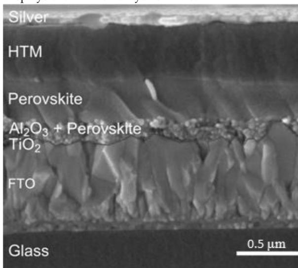
Figure 1: Each intricate layer of a perovskite cell as viewed under a SEM. From the bottom up: Fluorine doped tin oxide (FTO), Titanium oxide, aluminium oxide with perovskite, perovskite, the holetransporting material (HTM) consisting of poly(triaryl amine) (PTAA) and finally the opaque back contact - silver.
