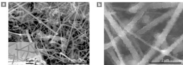
Figure 1: (Chan *et al.*) SEM images of pristine SiNWs (A) before and (B) after cycling of the battery. The images show the resilience of SiNWs to pulverisation during the lithiation process.
