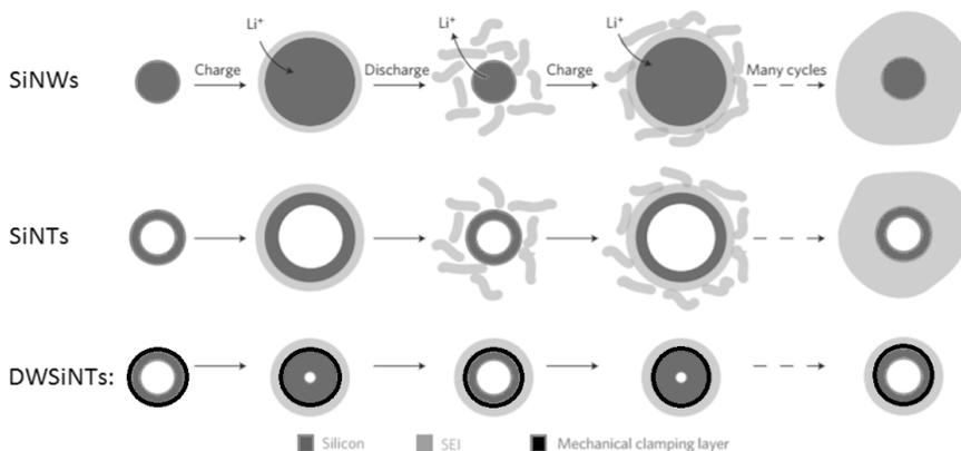
Figure 2: The formation of SEI around SiNWs SiNTs and DWSiNTs. Build up of SEI around SiNWs and SiNTs is a result of repeated expansion and contraction, whereas the outer wall of DWSiNTs maintains the same size and thus keeps the SEI layer thin.
