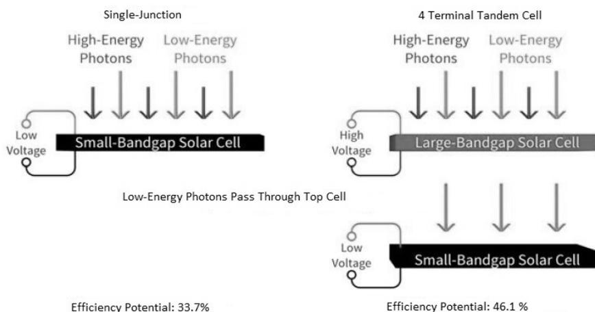
Figure 3: A comparison of theoretical max efficiencies for a single-junction and tandem solar cell is seen in this figure. Although the single-junction cell is capable of capturing both high-energy and low-energy photons due to its low bandgap it does so at a much lower voltage than the tuned large band gap tandem solar cell. Increased voltage means higher energy output with a theoretical increase of 12.4%.
