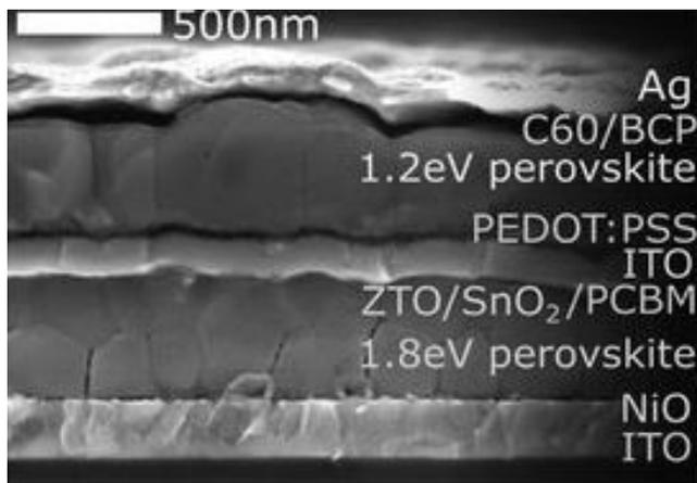
Figure 4: SEM image of a perovskite-perovskite tandem solar cell. Note the tuned bandgaps of the upper and lower perovskite layers. From the bottom up we see indium tin oxide (ITO), Nickel Oxide, a 1.8eV perovskite layer, a combined Zinc tin oxide (ZTO), Tin Oxide and phenyl-C<sub>61</sub>-butyric acid methyl ester (PCBM) layer, ITO, poly(3,4-ethylenedioxythiophene) (PEDOT:PSS), a 1.2eV perovskite layer, C60 with bathocuproine (BCP) and finally the opaque silver back contact.
