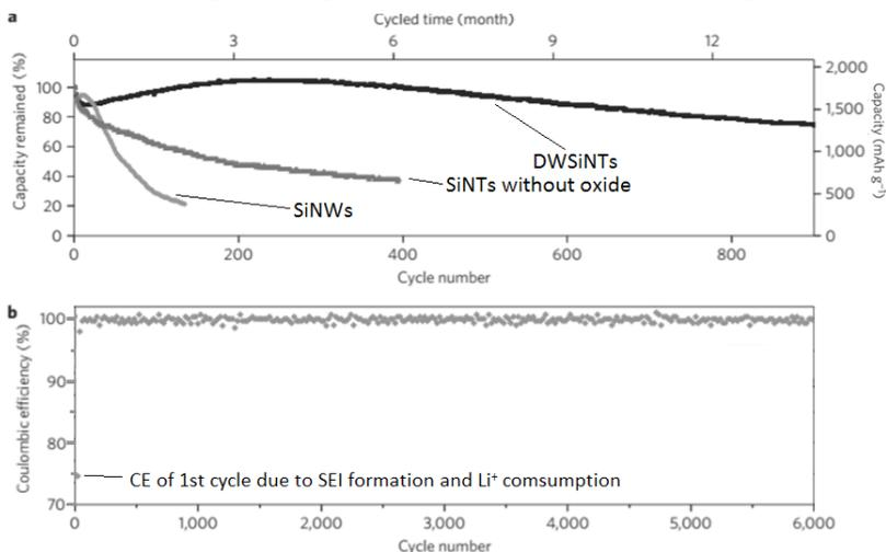
Figure 3: (A) The capacity of DWSiNTs, SiNTs and SiNWs at C/5. The latter two were shown to degrade considerably faster than DWSiNTs. The relatively large decrease of DWSiNTs was possibly due to electrolyte leakage over the 12 months that the experiment was run. (B) CE of DWSiNTs cycled at 12 C over 6000 cycles.
