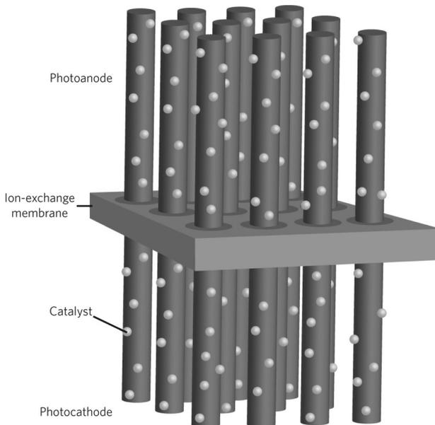
Figure 2: Dual microwire array. A tandem cell composed of a photoanode (which absorbs blue light and effects water oxidation), a photocathode (which absorbs red light and effects water reduction), and a polymeric membrane which separates the products and allows for the transfer of ions. The photoelectrodes are decorated with electrocatalysts.
