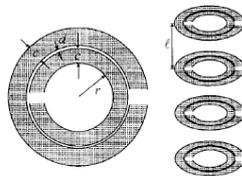
Figure 1: (A) overhead view of the SRR system (B) stacking sequence of the SRR array. Adopted from Pendry *et al.*<sup>4</sup>
