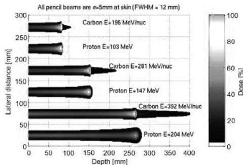
Figure 4. Dose distribution comparison of proton and carbon ion beams. Note the fragmentation tail, and increased dose at peak for the carbon beams (Suit *et al.*, 2010).
