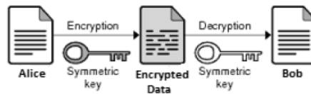
Figure 2. (Adapted from Skelton, 2015) Symmetric key encryption. Both the sender and receiver are in possession of the same key and use this to encrypt and decrypt the message.
